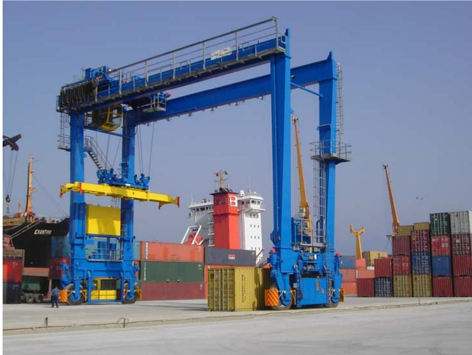
Fig 11- Rubber Tyre Gantry
