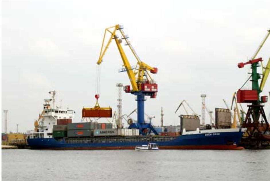
Fig 6-Multipurpose Slewing Crane
