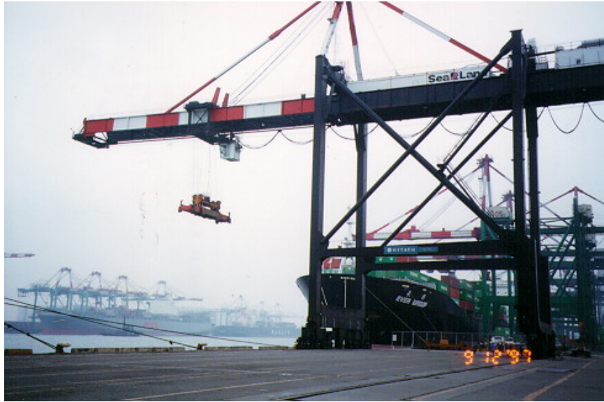
Hitachi Crane in Sealand, Kaohsiung before Span Change (24.38 metres)
